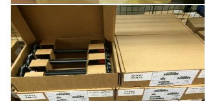
Dividers allow access to multiple parts. Reduces part extraction time and excess materials.
